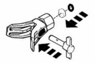
Thread the paint hose back onto the spray gun. Tighten with a wrench.
