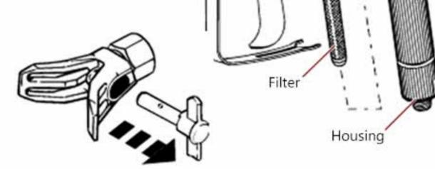
Clean spray tip and filter with a soft-bristled brush and the appropriate cleaning solution. Be sure to remove and clean the washer and saddle seat located in the rear of the spray tip assembly.
